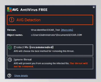
If **AVG AntiVirus Free Edition** fails to identify the EICAR test file as a virus, you should check the program configuration again!
